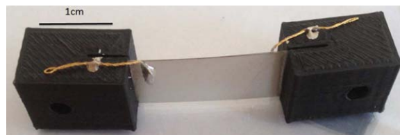
Figure 2. Sample mounted in clamps with attached electrodes for piezoelectric strain measurements. [Color figure can be viewed in the online issue, which is available at wileyonlinelibrary.com .]
